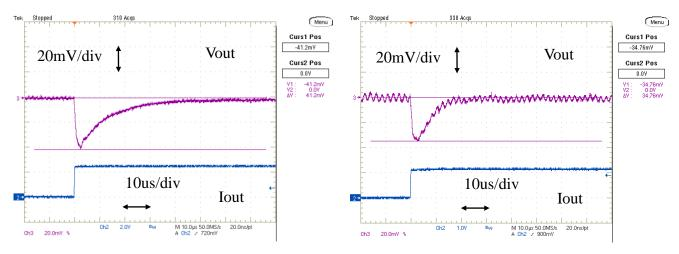
Fig. 12-1a. Load Transient Response (MPDRX301S)
