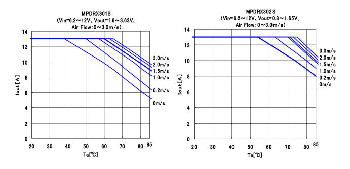
The above derating limits apply to this product soldered directly to 101.6\*180mm\*1.6mm PCB (6 layer). Any adjacent parts of high temperature may cause overheating. For reliable operation, please ensure that the FET temperature of this product is maintained below 120°C and the inductor temperature is below 111°C.
