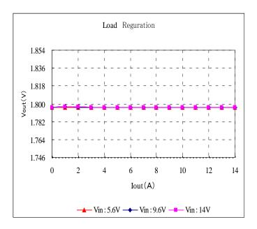
Fig. 12-3-7. Output Voltage v.s. Output Current
