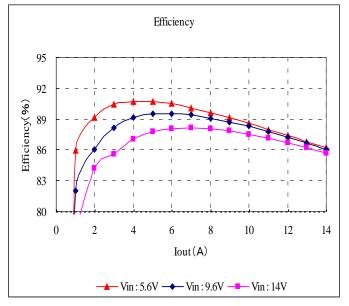
Fig. 12-3-8. Efficiency v.s. Output Current
