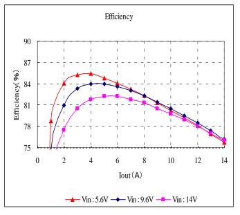
Fig. 12-3-17. Efficiency v.s. Output Current
