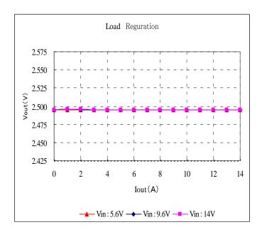
Fig. 12-3-4. Output Voltage v.s. Output Current
