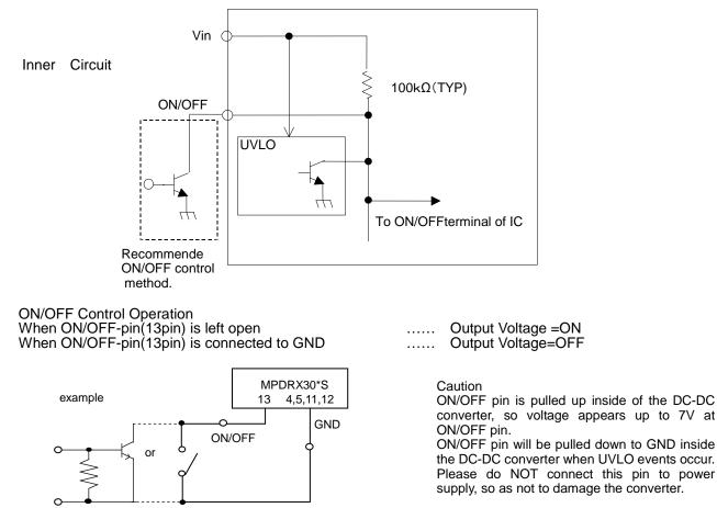
ON/OFF pin of MPDRX301S/302S/303S/304S can be connected each other. The maximum number is up to 20pcs.
