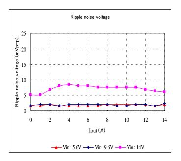
Fig. 12-3-12. Ripple Voltage v.s. Output Current
