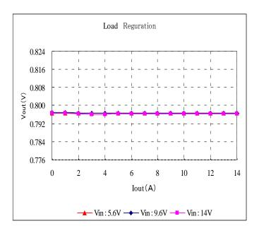
Fig. 12-3-16. Output Voltage v.s. Output Current
