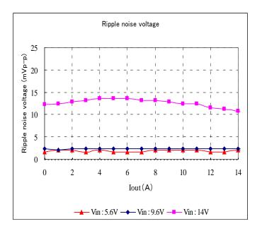
Fig. 12-3-6. Ripple Voltage v.s. Output Current
