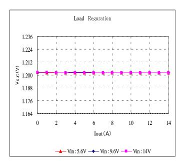
Fig. 12-3-13. Output Voltage v.s. Output Current
