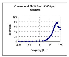
Fig. 12-2-2. Output Impedance of conventional product
