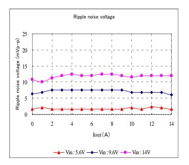
Fig. 12-3-18. Ripple Voltage v.s. Output Current
