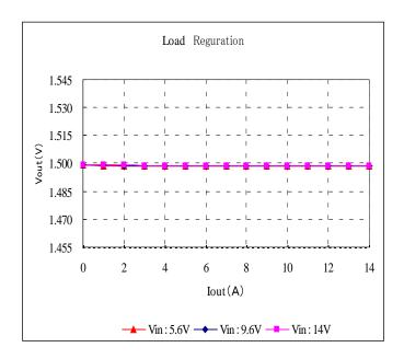
Fig. 12-3-10. Output Voltage v.s. Output Current
