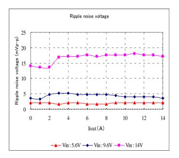
Fig. 12-3-9. Ripple Voltage v.s. Output Current
