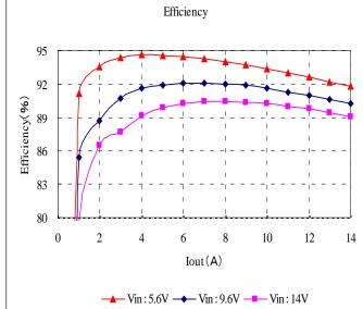
Fig. 12-3-2. Efficiency v.s. Output Current
