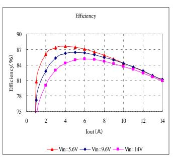
Fig. 12-3-14. Efficiency v.s. Output Current
