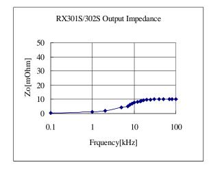
Fig. 12-2-1. Output Impedance of MPDRX301S/302S
