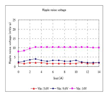
Fig. 12-3-15. Ripple Voltage v.s. Output Current
