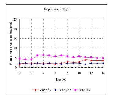
Fig. 12-3-3. Ripple Voltage v. s. Output Current
