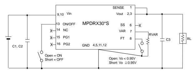
$\begin{array}{c} C1,C2:10\mu F \diagup 25V \ (Ceramic Capacitor) \\ C3:100\mu F \backsim 6.3V \ (Ceramic Capacitor) \\ \ref{eq:constraint} \ref{eq:constraint}$
