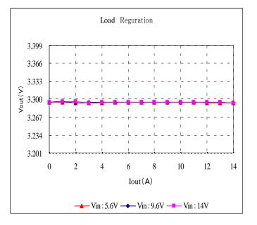
Fig. 12-3-1. Output Voltage v.s. Output Current
