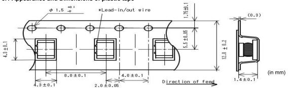
Dimension of the Cavity is measured at the bottom side.
