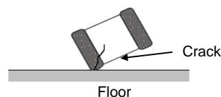
3. When printed circuit boards are piled up or handled, the corner of another printed circuit board should not be allowed to hit the capacitor in order to avoid a crack or other damage to the capacitor.
