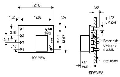
[unit: mm] Tolerance: 0.25mm
