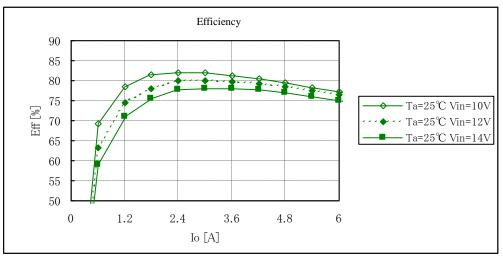
Fig. 12-1-2. Efficiency v. s. Output Current
