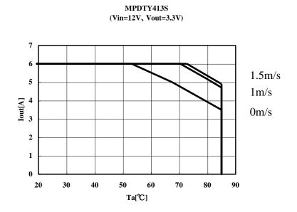
When using this product at the ambient air temperature of 55°C more, it is used by the following temperature derating.
