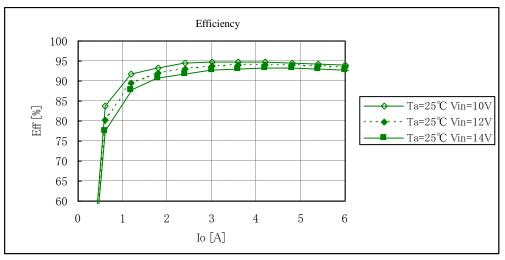
Fig. 12-2-2. Efficiency v. s. Output Current
