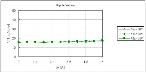
Fig. 12-1-3. Ripple Voltage v. s. Output Current
