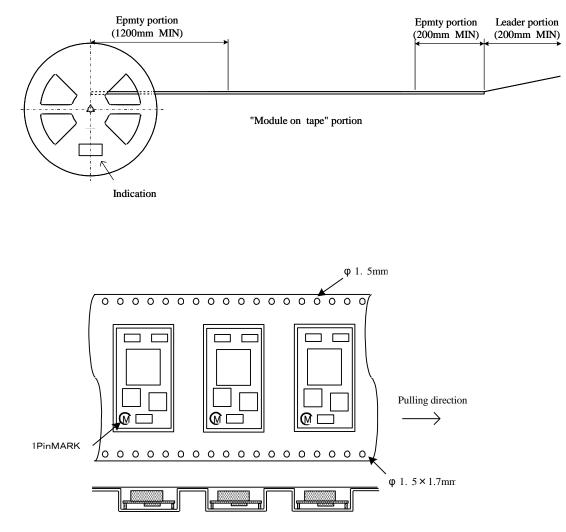
The module is located such as inductor in upper side and terminal in lower side.
