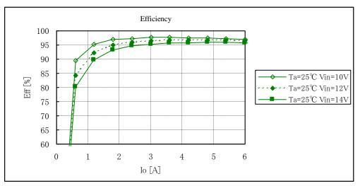
Fig. 12-3-2. Efficiency v. s. Output Current
