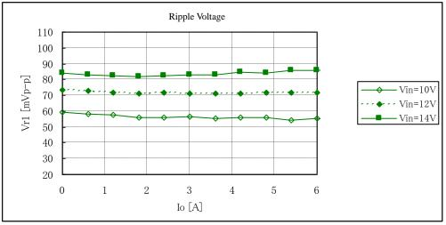
Fig. 12-3-3. Ripple Voltage v. s. Output Current
