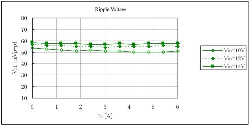
Fig. 12-2-3. Ripple Voltage v. s. Output Current
