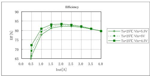
Fig. 12-2-11. Efficiency v. s. Output Current
