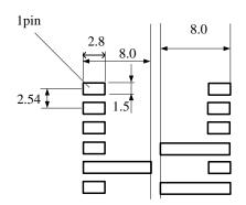
There are wiring coppers or through-hole via at the bottom side of the DC-DC converter. When you design your PCBs, please be careful not to short the circuit of the DC-DC converter or PCBs.
