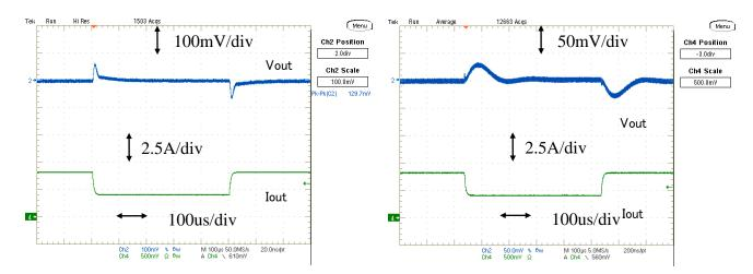
Fig. 12-1a. Load Transient Response (Cout: 0uF)
