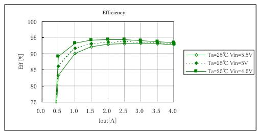
Fig. 12-2-2. Efficiency v. s. Output Current
