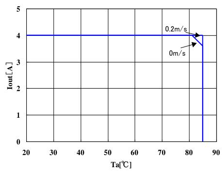
The above derating limits apply to this product soldered directly to 101.6\*180mm\*1.6mm PCB (double-sided, with 70um copper). Any adjacent parts of high temperature may cause overheating. For reliable operation, please ensure that the FET temperature of this product is maintained below 120°C and the inductor temperature is below 106°C.
