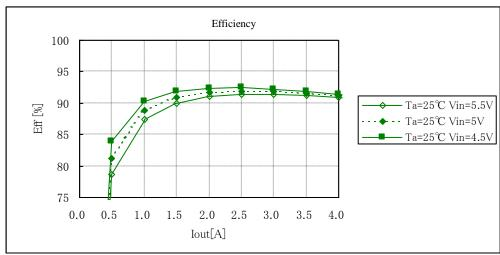
Fig. 12-2-5. Efficiency v. s. Output Current
