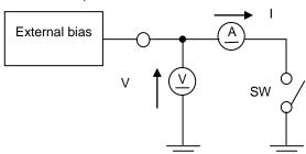
External bias voltage shall be measured when SW left open.
