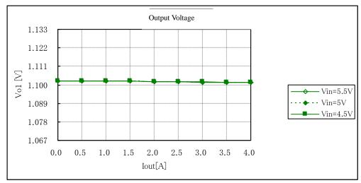
Fig. 12-2-7. Output Voltage v.s. Output Current
