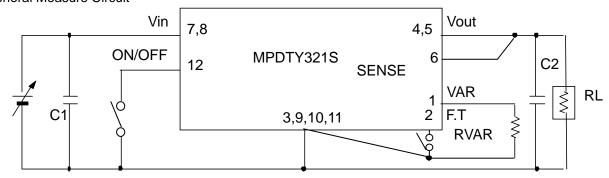
C1 :  $22\mu F/10V$  Ceramic Capacitor C2 :  $47\mu F/6.3V$  Ceramic Capacitor
