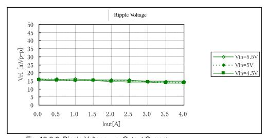
Fig. 12-2-9. Ripple Voltage v. s. Output Current
