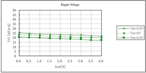
Fig. 12-2-6. Ripple Voltage v. s. Output Current
