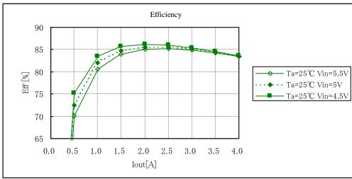
Fig. 12-2-8. Efficiency v. s. Output Current
