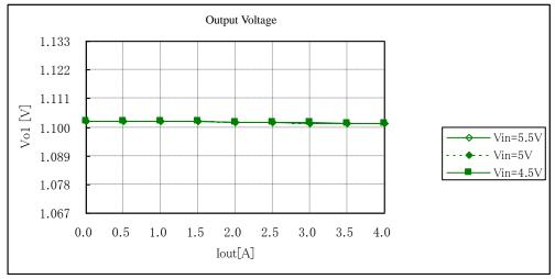
Fig. 12-2-1. Output Voltage v.s. Output Current
