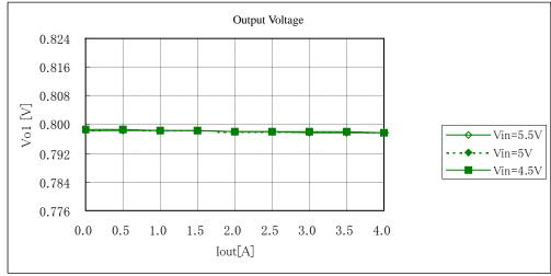
Fig. 12-2-10. Output Voltage v.s. Output Current
