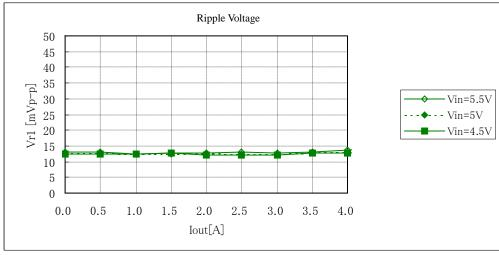
Fig. 12-2-12. Ripple Voltage v. s. Output Current
