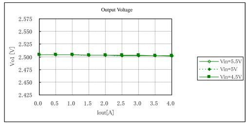
Fig. 12-2-4. Output Voltage v.s. Output Current
