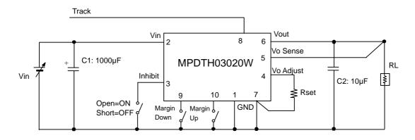
$\begin{array}{lll} \text{C1} & : & 1000 \mu \text{F}/25 \text{V} & (\text{Aluminum Electrolytic Capacitor}) \\ \text{C2} & : & 10 \mu \text{F}/6.3 \text{V} & (\text{Ceramic Capacitor}) \\ \end{array}$
