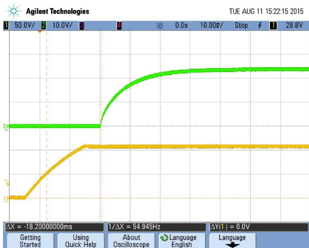
Turn-on transient at zero load current (10 mS/div, Top Trace: Vout, 10V/div; Bottom Trace: Vin, 50V/div)
