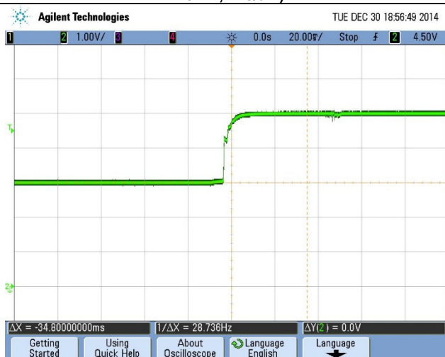
Start-up into a Pre-bias Load@25°C
