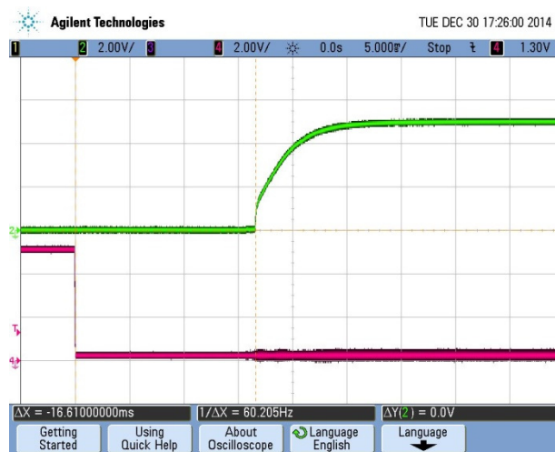
Turn-on transient at full load current (5 mS/div, Top Trace: Vout, 2V/div; Bottom Trace: ON/OFF, 2V/div)
