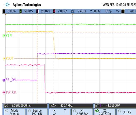
Figure 10: Turn-off by PS_ON Delay: Back
