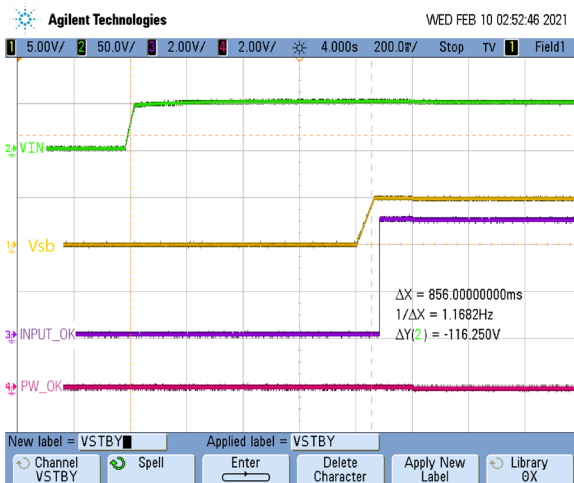
Figure 7: Turn-on Delay; Vin to Vsb delay: back
