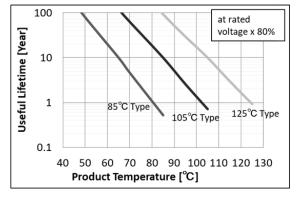
Murata's General MLCC products are designed for use in devices with a typical lifetime around 10 years. Murata's general MLCC products are designed so that the useful lifetime can be extended longer than 10 years under the following conditions: [80% of the rated voltage or less, Maximum operating temperature -20 degree C or less] Extended useful lifetime, under specific operating conditions, can be estimated from the chart.
