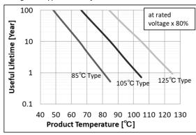
Murata's General MLCC products are designed for use in devices with a typical lifetime around 10 years.
