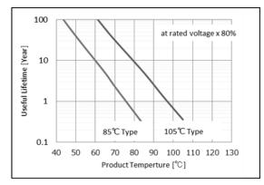
These MLCC products are designed for use in devices with a typical lifetime of less than 5 years.
