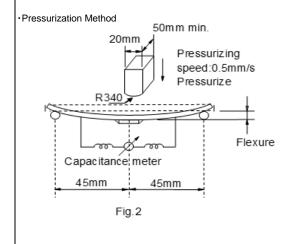
**Except for Substrate Bending test**
