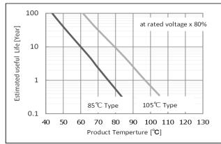
These MLCC products are designed for use in devices with a typical lifetime of less than 5 years.
