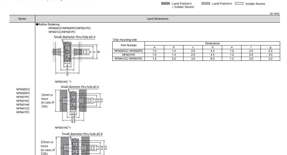
\*1 For large current design, width of signal land pattern should be wider not less than 1mm per 1A (1mm/A). For example, in case of 10A, signal land pattern width should be 10mm or more. (1mm/A\*10A=10mm)
