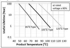
Murata's General MLCC products are designed for use in devices with a typical lifetime around 10 years.
