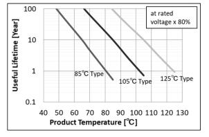
Murata's General MLCC products are designed for use in devices with a typical lifetime around 10 years. Murata's general MLCC products are designed so that the useful lifetime can be extended longer than 10 years under the following conditions: [80% of the rated voltage or less, Maximum operating temperature -20 degree C or less] Extended useful lifetime, under specific operating conditions, can be estimated from the chart.
