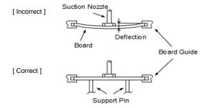
2. Dirt particles and dust accumulated in the suction nozzle and suction mechanism prevent the nozzle from moving smoothly. This creates excessive force on the capacitor during mounting, causing cracked chips.
