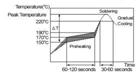
[ Standard Conditions for Reflow Soldering ]
