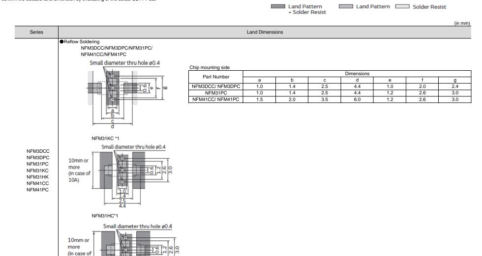
\*1 For large current design, width of signal land pattern should be wider not less than 1mm per 1A (1mm/A). For example, in case of 10A, signal land pattern width should be 10mm or more. (1mm/A\*10A=10mm)
