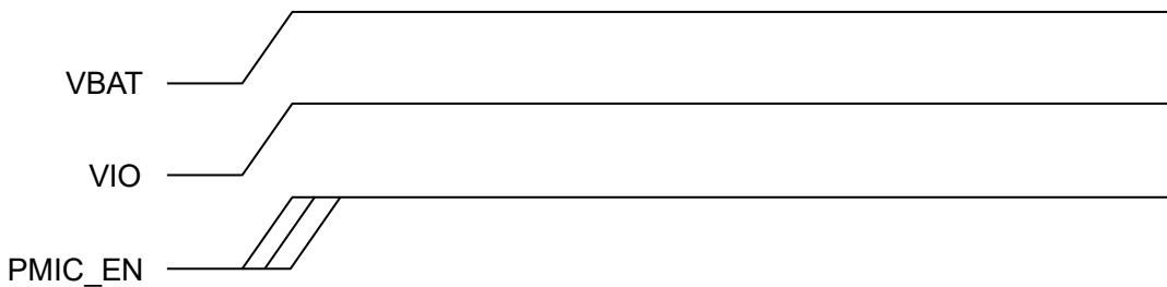
A minimum time of 100ms is required after PMIC\_EN is deasserted (=0) and before it is asserted (=1).
