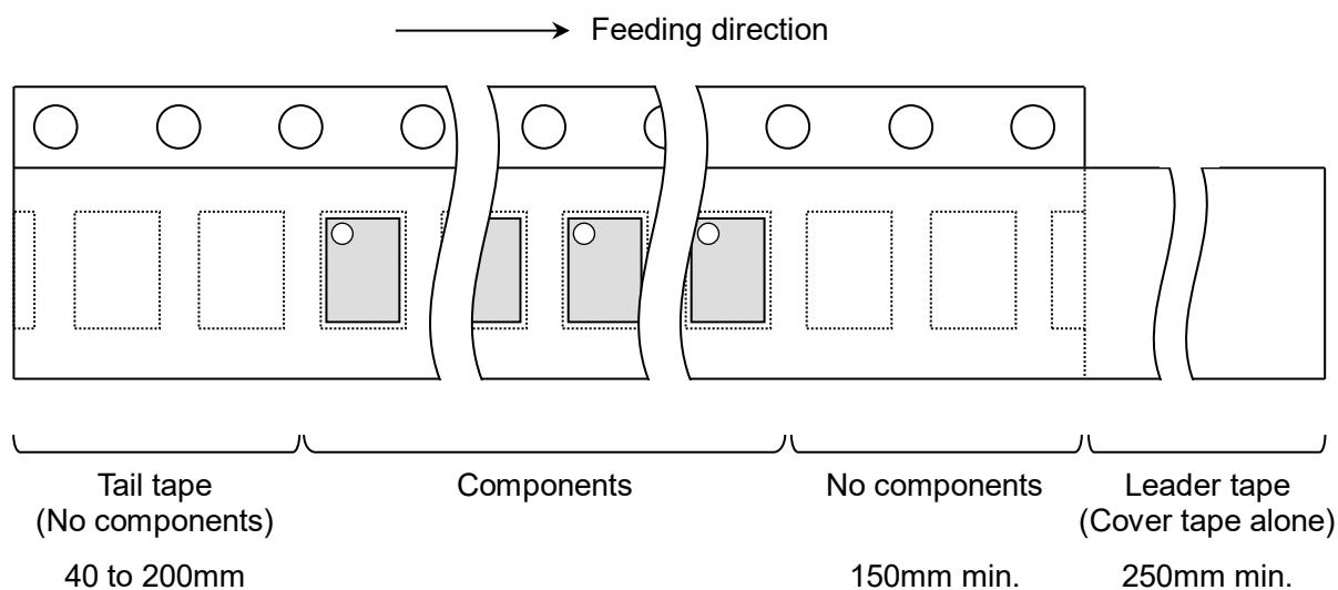
(5) The tape for chips are wound clockwise, the feeding holes to the right side as the tape is pulled toward the user.
