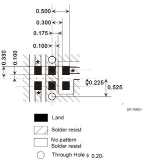
\*Line width to be designed to match  $50\Omega$  characteristic impedance, e depending on PCB material and thickness. e
