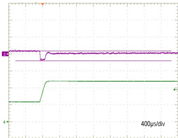
Start-up ( V_{in}=48V , V_{out}=5V , I_{out}=12A , T_a=+25^{\circ}C ) Ch1=Vin, 50V/div, Ch2=Vout, 2V/div.
