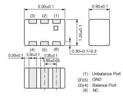
\* Terminal of "NC" should be connected the floating land. \* All the technical data and information contained herein are subject to change without prior notice. (in mm)
