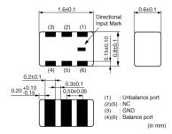
\*Terminal of "NC" should be fixed to the no connected pattern All the technical data and Information contained herein are subject to change without prior notice.
