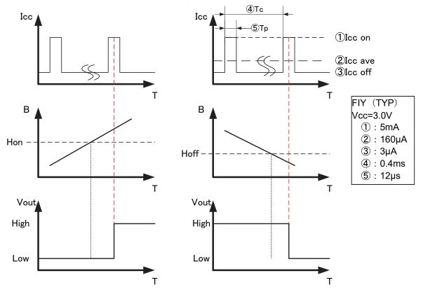
NOTE1) AMR element is driven by the intermittent switch curcuit shown in item 3-2. The timing of Vout change is subject to the period of Icc on.
