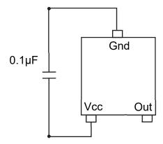
\* 0.1 μF is the recommended value and does not guarantee operation. Please select the suitable capacity depending on the usage environment. In addition, when the sensor is used under high noise level, Zener diode is recommended in parallel with a bypass capacitor.
