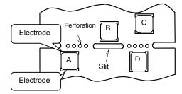
(3) Mounting components near screw holes
