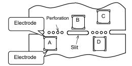
(3) Mounting components near screw holes
