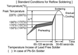
[Allowable Reflow Soldering Temperature and Time]
