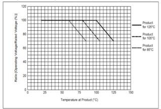
Derated products\*1 are suitable for use in circuits where continuous applied voltage and temperature to the capacitor is derated (below rated voltage and temperature). A reliability assurance level equivalent to standard products \*2 can be secured by restricting the voltage and temperature according to the derating conditions in the chart.
