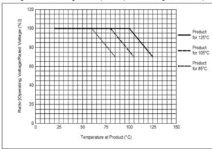
Derated products\*1 are suitable for use in circuits where continuous applied voltage and temperature to the capacitor is derated (below rated voltage and temperature). A reliability assurance level equivalent to standard products \*2 can be secured by restricting the voltage and temperature according to the derating conditions in the chart.
