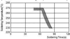
In the case of repeated soldering, the accumulated soldering time must be within the range shown above.
