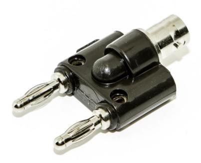
The BU-P1269 is a dual stacking 4mm banana plug to female BNC. Allows a BNC male connector to be converted for use with standard 4mm banana jacks spaced 0.75" center-to-center.
