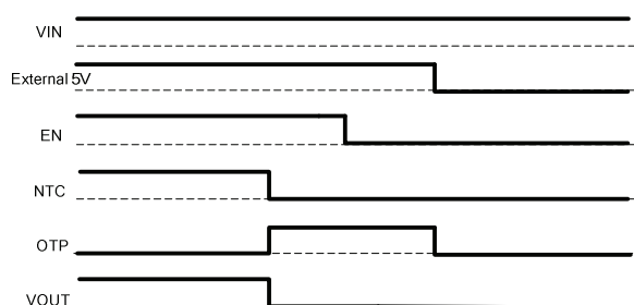
Figure 4: Normal Mode → NTC protection Mode → Transportation Mode
