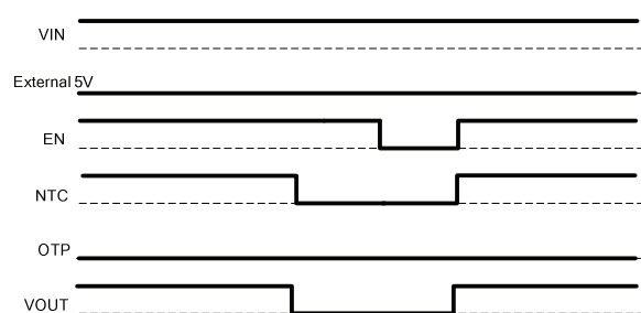
Figure 3: Normal Mode without external 5V → NTC protection Mode → EN Restart
