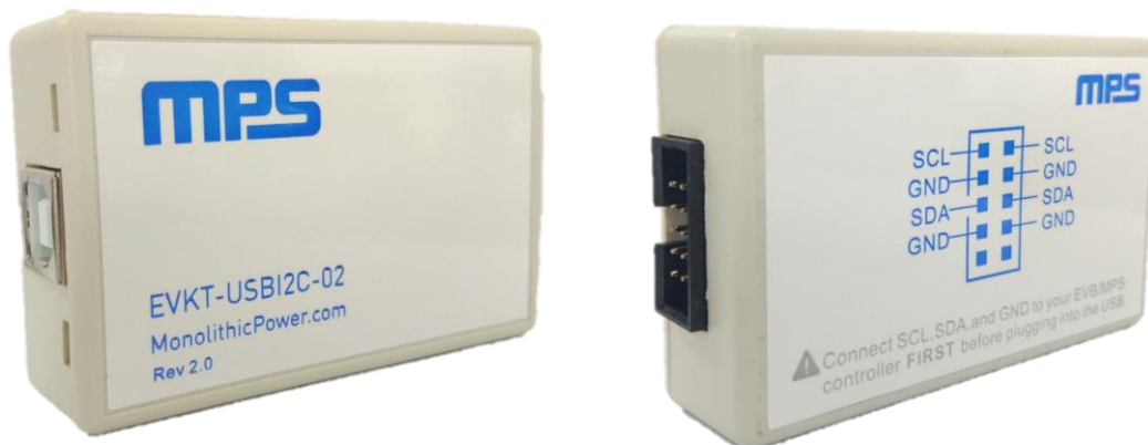
Figure 3: EVKT-USBI2C-02 Communication Interface Device
