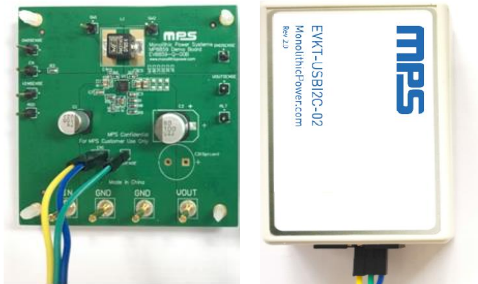
Figure 6: EVB to MPS I 2 C Communication Interface Device Wire Connection
