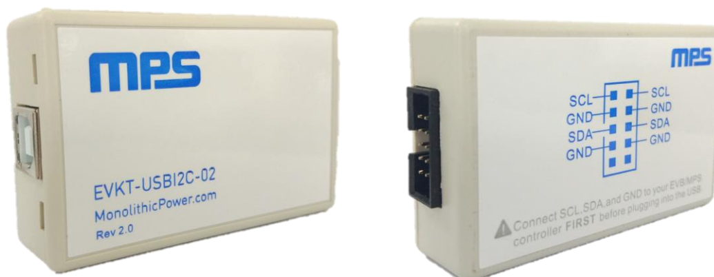
Figure 3: EVKT-USBI2C-02 Communication Interface Device
