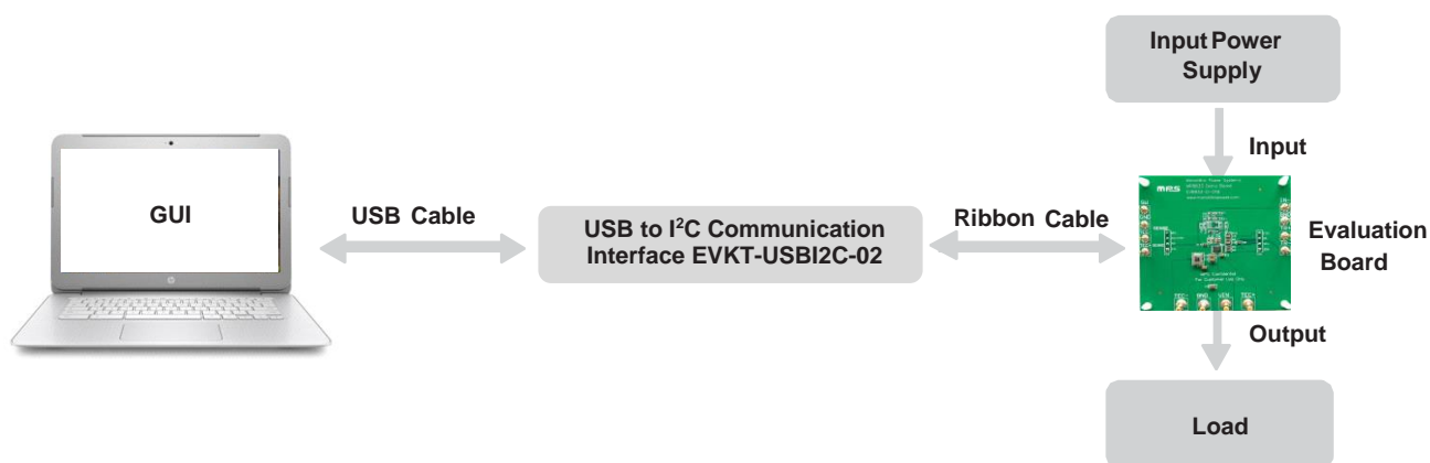
Figure 1: EVKT-MP8833 Evaluation Kit Set-Up
