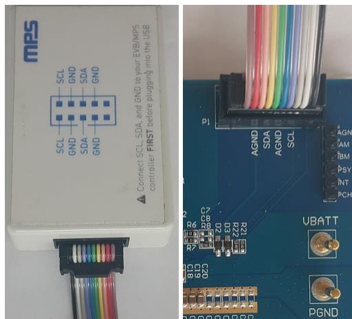
Figure 6: EVB to MPS I 2 C Communication Interface Wire Connection
