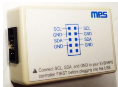
Figure 3: EVKT-USBI2C-02 Communication Interface
