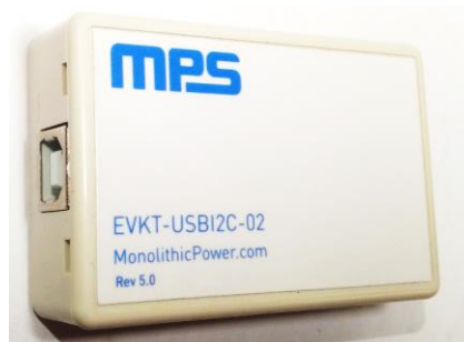
Figure 3: EVKT-USBI2C-02 Communication Interface
