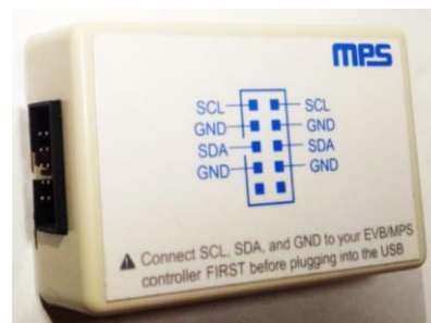
Figure 3: EVKT-USBI2C-02 Communication Interface
