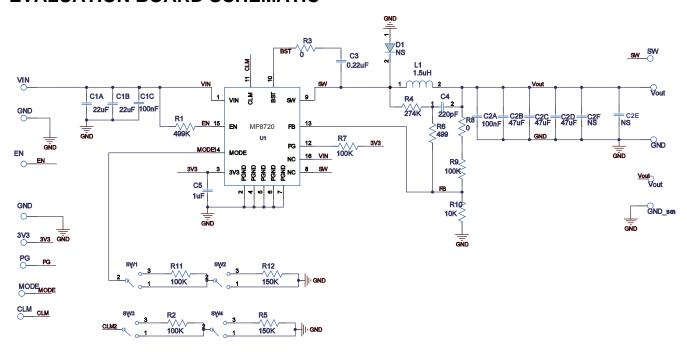
$V_{IN}$ =6-24V,  $V_{OUT}$ =5V,  $I_{OUT}$ =10A,  $f_{SW}$ =700kHz
