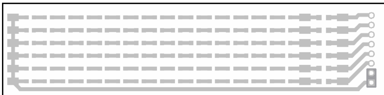
Figure 2—LED Board Top Layer
