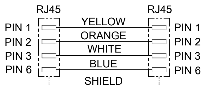
WIRING DIAGRAM FOR CABLE TYPE 11, 12
