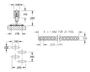
Interconnect Socket Surface Mount Socket Accepts .015"- .025" (0,38 - 0,635 mm) dia leads Single Row Surface Mount **Plating Code:** 43 Shell Plating: 200 µ" Tin (matte finish) over 100 µ" Nickel Inner Contact Plating: 30 µ" Gold over 50 µ" Nickel
