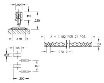
Interconnect Socket Surface Mount Socket Accepts .015"- .025" (0,38 - 0,635 mm) dia leads Single Row Surface Mount **Plating Code:** 43 Shell Plating: 200 µ" Tin (matte finish) over 100 µ" Nickel Inner Contact Plating:
