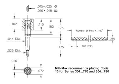
**Description:** Interconnect Socket Solderless Press-Fit Socket Accepts .015"- .025" (0,38 - 0,635 mm) dia leads Single Row Through Hole Plating Code: Shell Plating:
