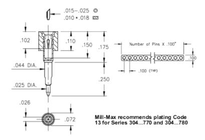
**Description:** Interconnect Socket Solderless Press-Fit Socket Accepts .015" - .025" (0,38 - 0,635 mm) dia leads Single Row Through Hole **Plating Code:**
