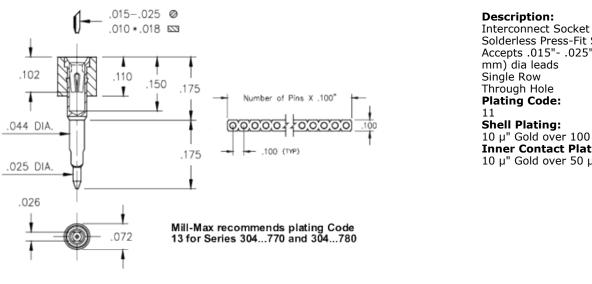
Solderless Press-Fit Socket Accepts .015"- .025" (0,38 - 0,635 mm) dia leads Single Row Through Hole Plating Code: 11 Shell Plating: 10 µ" Gold over 100 µ" Nickel Inner Contact Plating: 10  $\mu$ " Gold over 50  $\mu$ " Nickel
