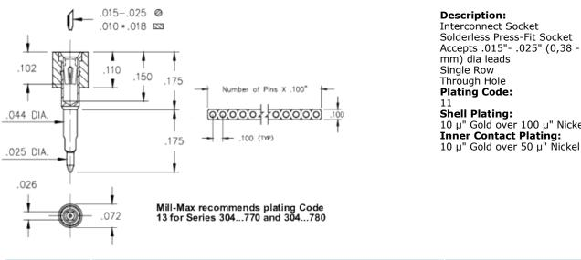
Interconnect Socket Solderless Press-Fit Socket Accepts .015"- .025" (0,38 - 0,635 mm) dia leads Single Row Through Hole Plating Code: 11 Shell Plating: 10 µ" Gold over 100 µ" Nickel Inner Contact Plating:
