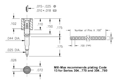
**Description:** Interconnect Socket Solderless Press-Fit Socket Accepts .015" - .025" (0,38 - 0,635 mm) dia leads Single Row Through Hole Plating Code:
