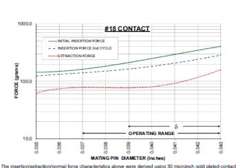
and polished steel gauge pins having a bullet-shaped tip. The curves represent typical average values; they are best used to compare the differences between similar size
