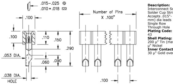
Interconnect Socket Solder Cup Strip Socket Accepts .015"- .025" (0,38 - 0,635 mm) dia leads Single Row Through Hole
