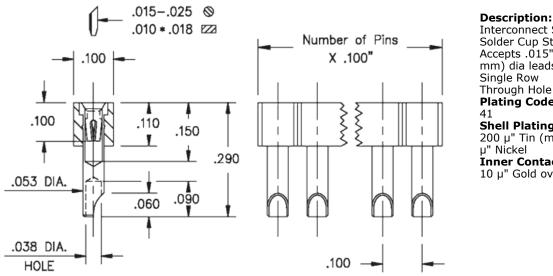
Interconnect Socket Solder Cup Strip Socket Accepts .015"- .025" (0,38 - 0,635 mm) dia leads Single Row Through Hole **Plating Code: Shell Plating:** 200 μ" Tin (matte finish) over 100 Inner Contact Plating: 10 μ" Gold over 50 μ" Nickel
